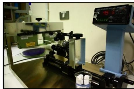
**Figure 4:** Facilities of hydrometer calibration - Diameter measurement unit
