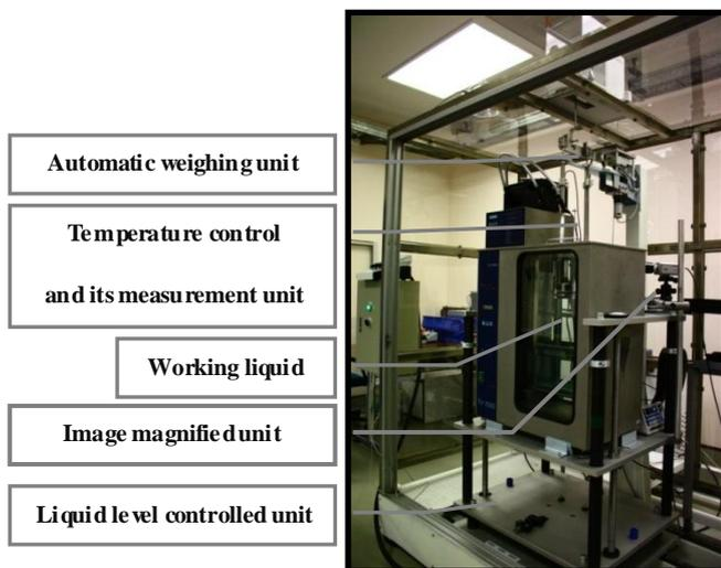
**Figure 3:** Facilities of hydrometer calibration- Hydrostatic weighing unit
