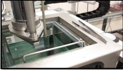
**Figure 5:** Density standard silicon ring is weighing in tri-tetradecane liquid
