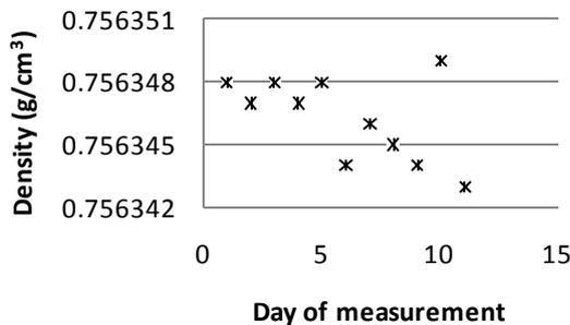
**Figure 6:** Density measurement results of Tri-tetradecane
