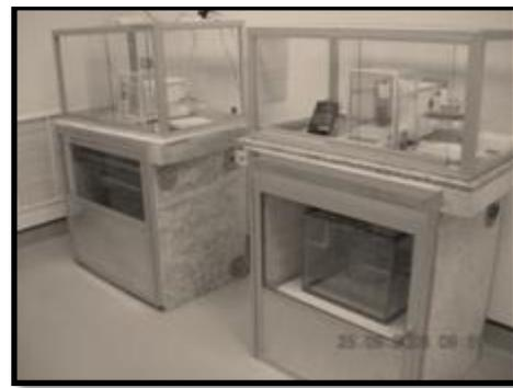
**Figure 1:** 1g-1kg OIML weight density measuring unit, water as a working fluid.
