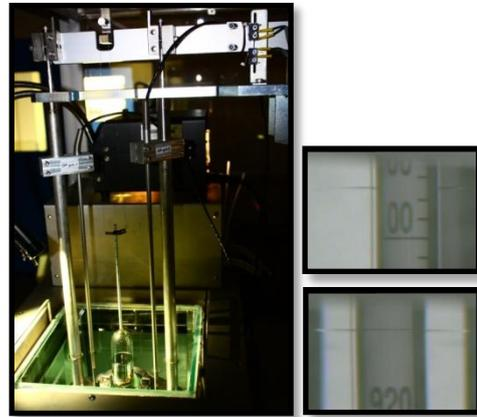
**Figure 7:** Hydrometer weighs in tri-tetradecane [Left]. Magnifying images of 0.2 kg/m³ scale division hydrometer from CCD camera [Right]
