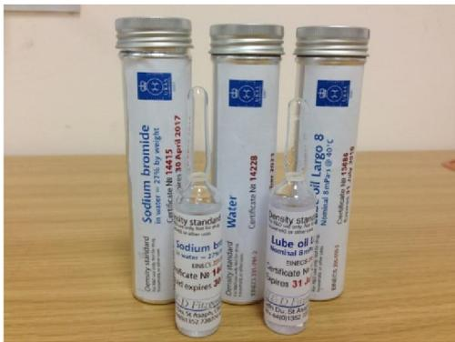
Figure 1. Standard liquids used for the calibrations of density meters.
