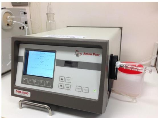
Figure 2. Density meter under test model DMA 5000 manufactured by Anton Paar.
